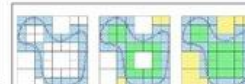
Figure 2: Constructing the quadtree of depth 4. Left: in a first step the quadtree is composed of blue cells (the boundary cells). Middle: classifying the empty leaf cells at depth 4. Green cells are inside the solid, yellow cells are outside the solid. Right: classifying the empty leaf cells at depth 4 - 1, i.e. 2.
